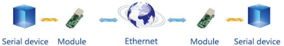
Manage multi serial client devices remotely via one web server:
