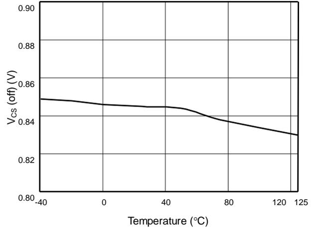
Fig. 8 V<sub>CS</sub> (off) vs. Temperature
