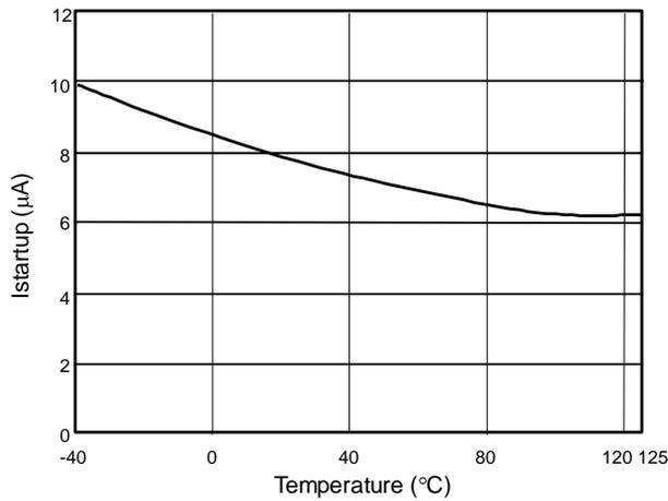
Fig. 9 Startup Current (I<sub>startup</sub>) vs. Temperature
